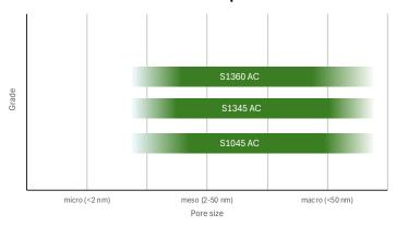
The "AC" series depth filter sheets are available in all standard sizes as well as in special cutouts. They are also available with covering safety paper (KP) both glued to the plate and inserted freely into the filtration device. The covering safety paper should prevent possible carbon leakage to the filtrate.
